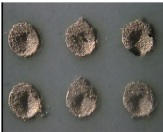
Fig. 6. Microscope view of the filled via holes that connect the third and fourth conductive layer.
